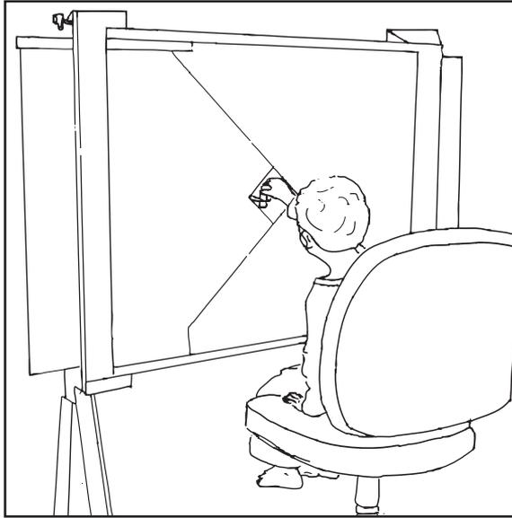
**Fig. 1.** Adjustable reaching apparatus. Participants sat on a swiveling office chair and reached through openings for targets. Between trials, participants faced away from the apparatus while it was adjusted. Infants sat on their caregiver's lap.
