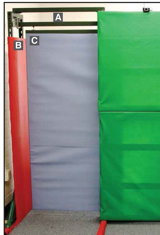
Fig. 1 Adjustable doorway apparatus. A free-standing metal frame (a) held a fixed wall (b) and a trolley on which a moveable wall (c) was mounted. The space between the two walls was adjusted to create doorways of varying width
