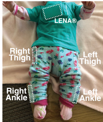
Figure 1. Sensor garment worn by infant participant. Four IMUs were placed in interior pockets sewn into a tightly-fitting pair of infant leggings. White dashed rectangles mark the approximate locations of each sensor pocket (above the left and right ankles and on the left and right thighs, just below the thighs). A white dashed rectangle also marks the LENA audio recorder worn in a pocket on the infant's shirt.
